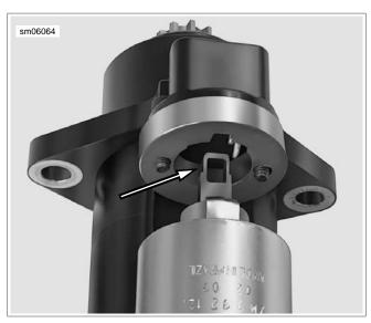
Figure 7-26. Capture Lever in Slot
