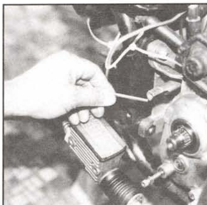
Be certain to install the spacers behind this mounting Hex before you grind for clearance.
