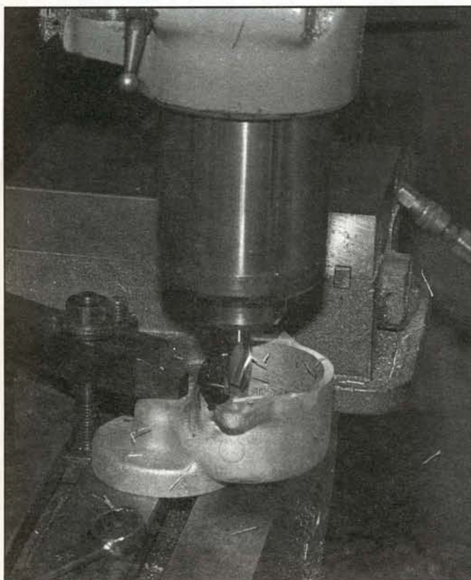
After welding, a mill is used to clearance drive.
