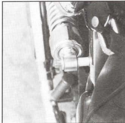
Shot of the top shock mount of Gail's 1989 Sportster. Early shock mounts demand different techniques to modify. Some harder, some easier.
