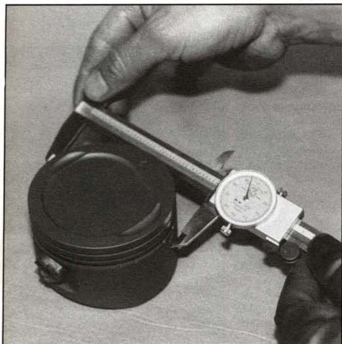
This is a photograph of a part that has been sprayed and baked with solid lubricant. The thickness of the coating can be as much as .0003, but burnishes down easily.
