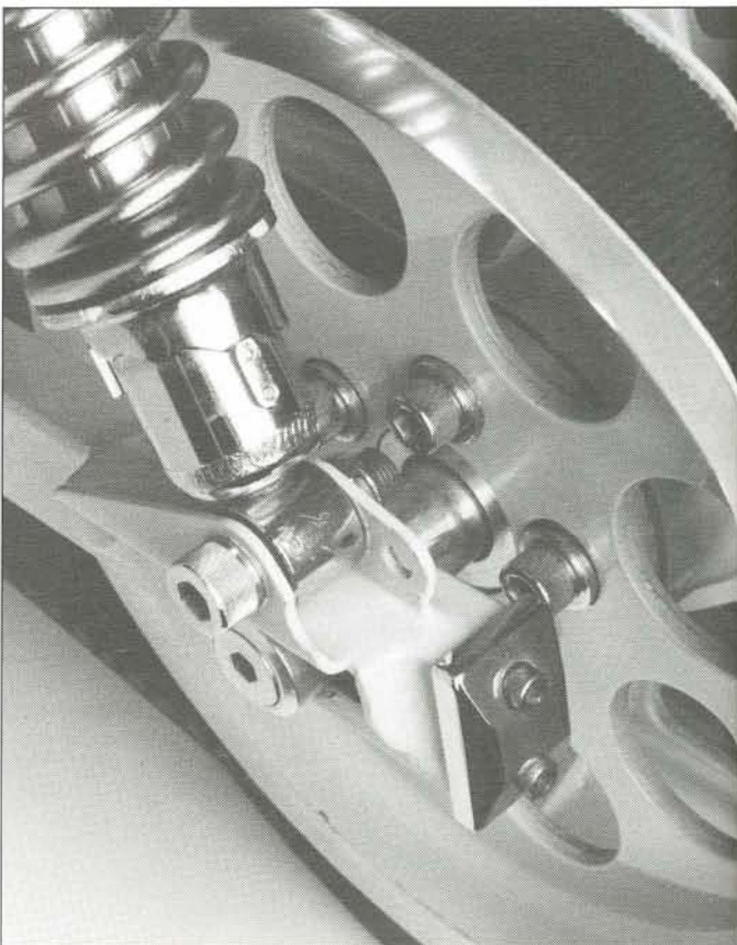
Had to machine a longer axle spacer and a piece to center the drive pulley with the wheel.
