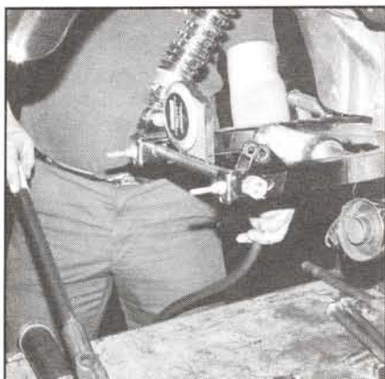
On the 1979 to 1983 models, the swingarm can be widened without being removed from the machine. Do not overheat.
