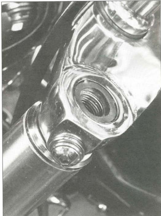
This is the special nut to adjust the neck bearings. Check adjustment again after the entire front end is assembled.
