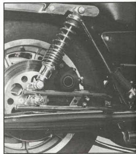
Carl's custom designed exhaust system with removable, adjustable baffles.
