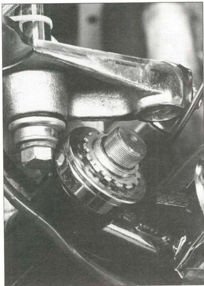
Common garden hose washers work perfectly to seal top-fork caps.
