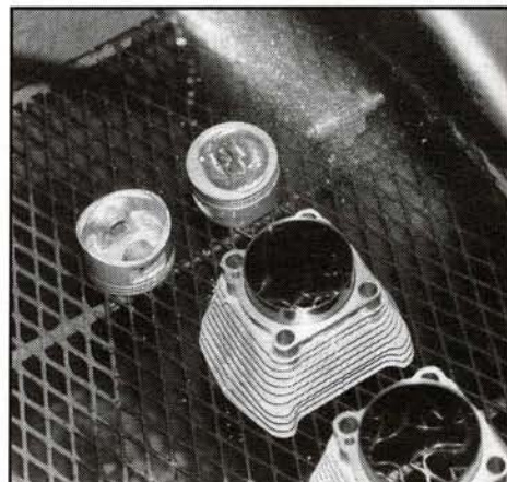
The most important procedure for proper bonding of solid lubrication is degreasing. Parts must be sprayed with clean solvents and scrubbed.
