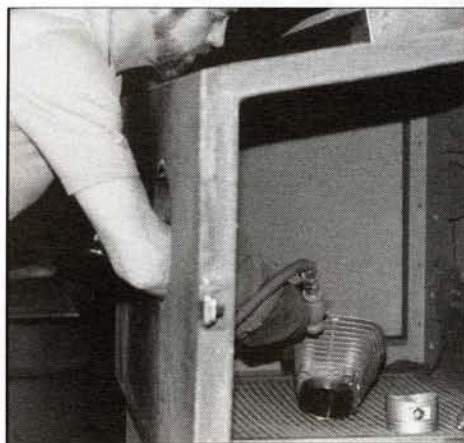
Sand blasting parts is necessary to remove or dislodge baked-on sludge and oil. Afterwards, parts need to be degreased again.
