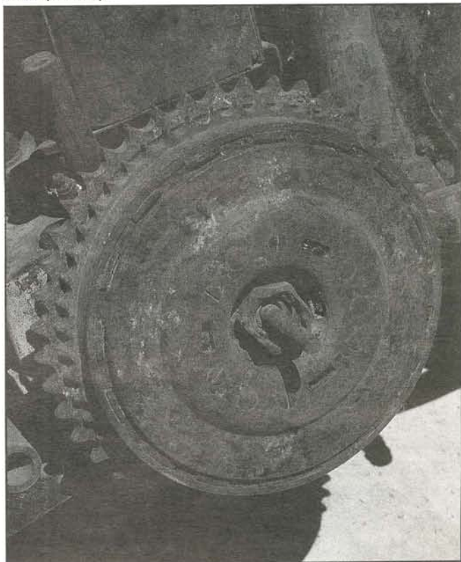
Cobble work to fix — an off-year clutch with the hub nut gouged out by a blunt chisel.
