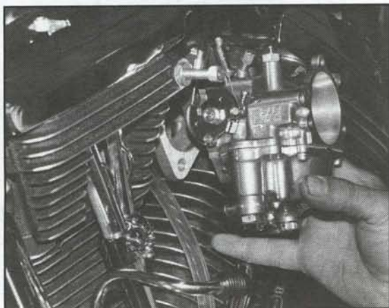
The new S&S shorty, E-series carb, with 1-7/8-inch venturi.
