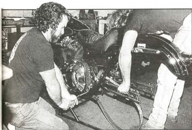
The engine/transmission must be aligned with the frame in order for the axle to be fed through the new swingarm.
