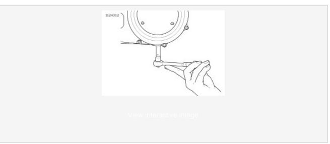
Figure 1. Removal/Installation of Chaincase Drain Plug
