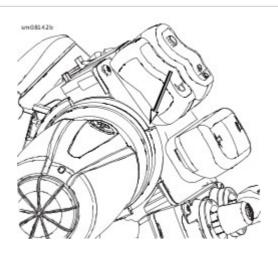
Figure 1. Sleeve Rubber Step to Switch Assembly Notch
