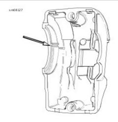
Figure 2. Glueless Grip Sleeve Locking Tooth
