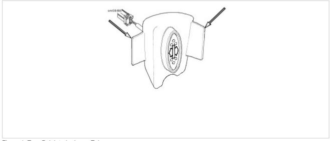
Figure 1. Tour-Pak Interior Lamp Tabs
