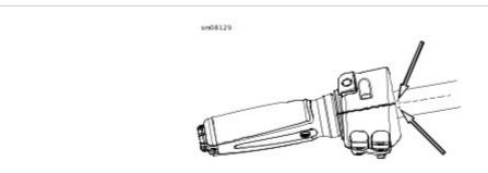
Figure 3. Alignment Dimples
